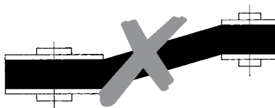
Axial misalignment of sheaves
