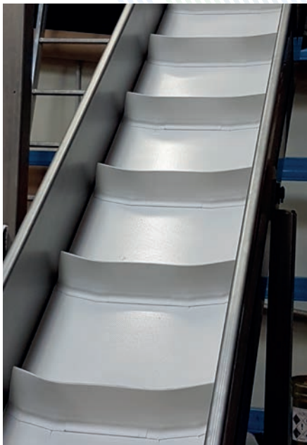
Belt with incurved cleats for inclined food conveying
